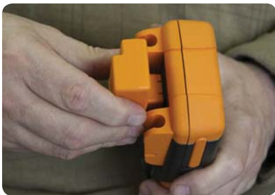
Figure 4: Attaching Agilent U1177A IR-to-Bluetooth adapter to the Handheld Multimeter
