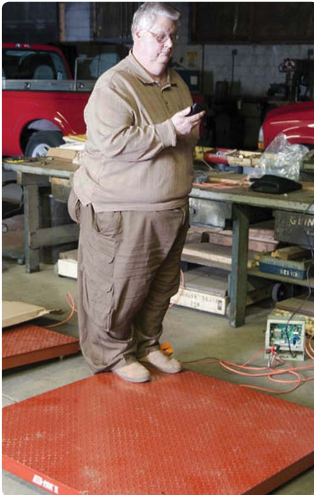
Figure 3. Identify a bad load cell with corner testing
